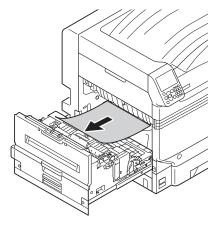
If there is remaining paper in the fuser unit then pull up the fuser unit's jam release lever (blue).
