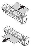
10 If the paper winds around the decal roller, remove the decal unit by turning the thumbscrews at both ends of the decal unit to the left, and remove the paper.
