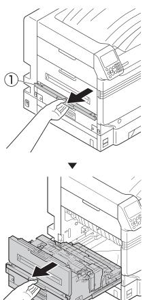
5 Check inside of the printer, and slowly remove the remaining paper.
