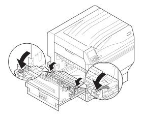
12 Set the fuser unit to the label position of the exit unit by holding its handle with your hands.
