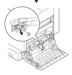
Firmly insert the new separation roller (③) along the notch, and mount the separator (④).
