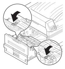
If there is no remaining paper in the fuser unit then pull up the fuser unit's lock lever (blue).
