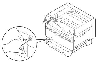
2 Check that the operation panel is completely turned off, and then switch off the main power supply.
