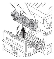
If a paper jam occurred in the fuser unit, raise the jam release lever (blue), and slowly pull the paper out in the opposite direction from the paper operation direction.
