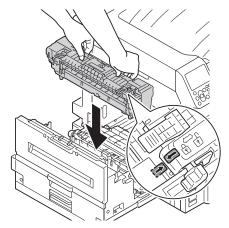
13 Push down the lock lever (blue) of the fuser unit.
