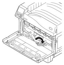
Rotate the belt unit left/right lock lever knob (blue) to the left, and push the lock lever towards yourself.
