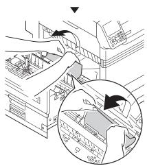
10 Hold the knob, push down the transfer roller unit.
