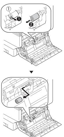
6 Lift Section A, release the claws in the direction shown in figure, and remove the paper feed rollers (2).
