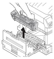
If the paper winds around the decal roller, remove the decal unit by turning the thumbscrews at both ends of the decal unit to the left, and remove the paper.
