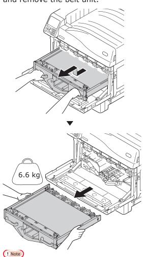
• Do not touch the belt surface or damage the belt.
