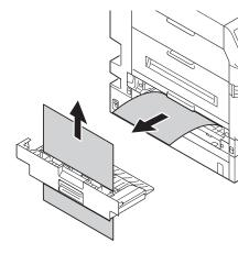
Put the 2-Sided Printing unit back into the printer.
