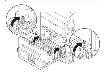
16 Hold the transfer roller unit's label part (blue) and remove it.
