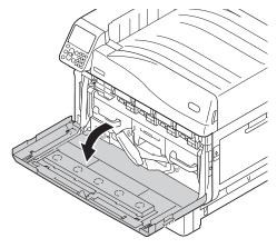
Remove the waste toner box from the printer.
