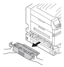
Remove the remaining paper from the printer.
