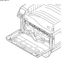
Gently lift the handle (blue) upwards, and remove the image drum taking care that your hand does not touch the drum on the lower side (green cylindrical section).
