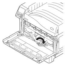
Rotate the belt unit left/right lock lever knob (blue) to the left, and push the lock lever towards yourself.
