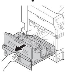
2 Check inside of the printer, and slowly remove the remaining paper.
