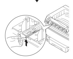
Apply an adhesive tape to hold the toner cartridge lever in the raised condition.
