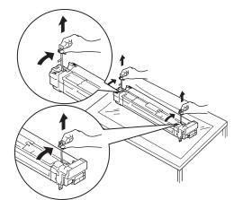
Align the image drum and arrow label (red) of printer, slowly insert in the slot taking care that your hand does not touch the photoreceptor (green) below, and firmly push it inside.
