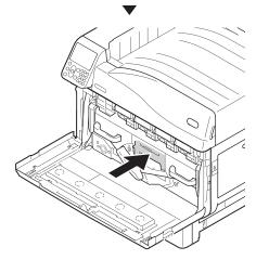
14 Align the image drum and arrow label (red) of printer, slowly insert in the slot taking care that your hand does not touch the photoreceptor (green) below, and firmly push it inside.
