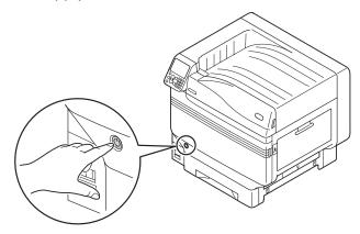
Check that the operation panel is completely turned off, and then switch off the main power supply.
