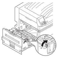
6 Hold the fuser unit handle with both hands, and remove it onto a flat surface.
