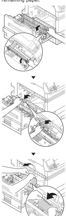
11 Hold the knob, push down the transfer roller unit.
