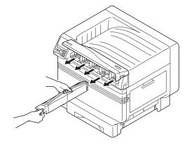
Check the toner cartridge detection levers (four levers for C911/C931/ES9411/ES9431/Pro9431, and five levers for C941/ES9541/Pro9541).
