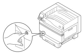
2 Check that the control panel has been turned off completely, and then turn off the main power.
