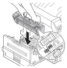
Push down the fuser unit's lock lever (blue).
