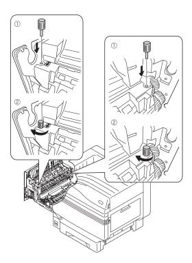
12 Hold the fuser unit handle with both hands, and set to the output unit.
