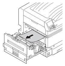
If the paper tip is not visible, pull up the fuser unit's lock lever (blue).
