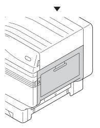
13 Switch on the main power supply, press the power supply switch and start the printer.
