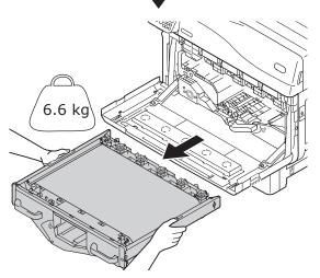
• Do not touch the belt surface or damage the belt.
