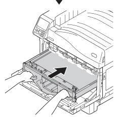
11 Raise the belt unit left/right lock lever, rotate the lock lever knob (blue) to the right and lock it.
