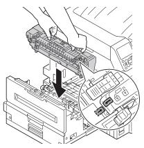
12 Push down the fuser unit's lock lever (blue).
