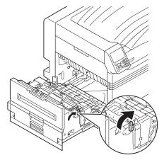
Hold the fuser unit handle with both hands, and remove it onto a flat surface.
