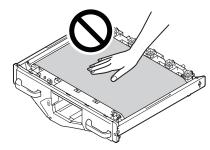
Removing the belt unit will expose all image drums to light. For preventing the optical deterioration of image drums, do not leave them as it is for more than 5 minutes after removing the belt unit.
