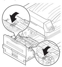
If there is no remaining paper in the fuser unit then pull up the fuser unit's lock lever (blue).
