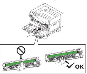
Remove the waste toner box from the printer.
