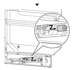
Insert the new feed rollers (1) in the axial, and firmly insert up to inside.
