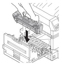
13 Push down the fuser unit's lock lever (blue).
